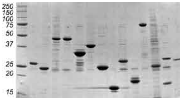
Figure 1: 14 Human proteins purified in soluble form from E. coli cells. Lane 1: size marker. SDS-PAGE and Coomassie staining.
